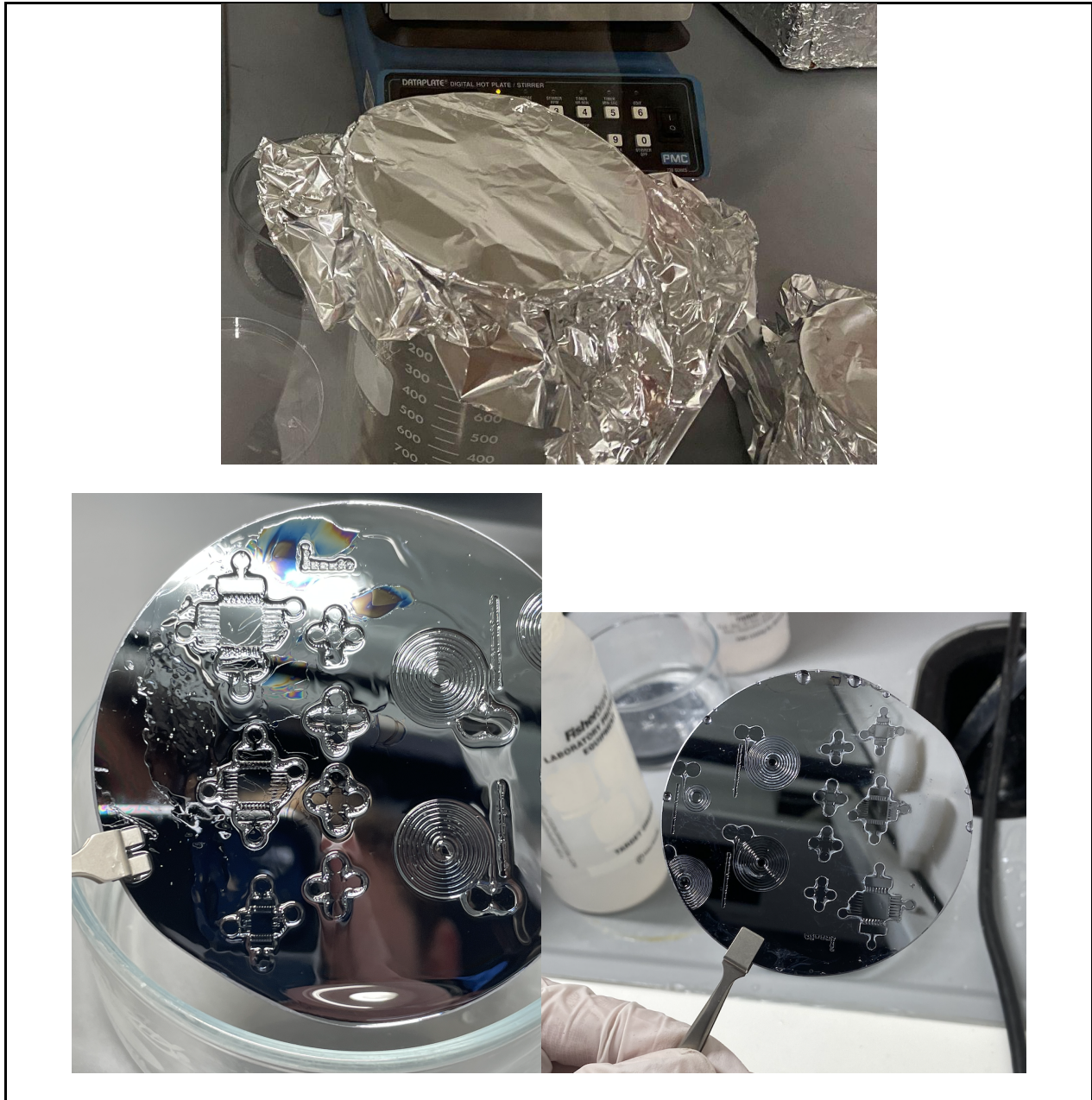
Figure 5: Development of the SU-8 coat on the wafer within an aluminum foil covered beaker (left), the resulting patterned SU-8-wafer following development (middle), and the final wafer product after isopropanol rinsing and nitrogen gas drying (right).
