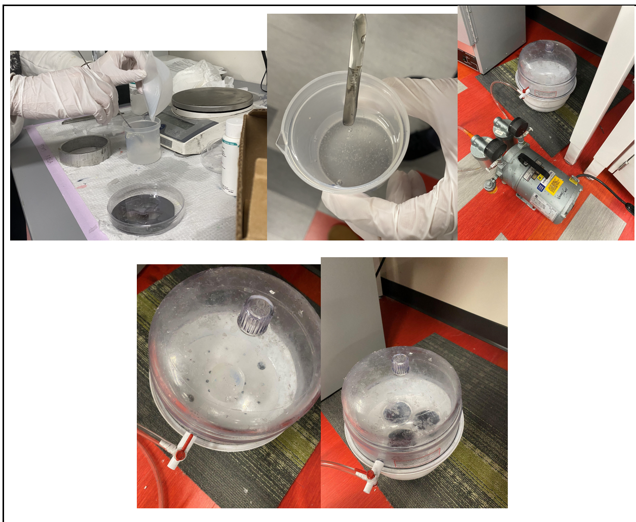
Figure 6: Preparation of the 10:1 ratio of Sylgard 184 silicone elastomer base and elastomer curing agent in order to generate the desired PDMS solution (top left) as well as a depiction of solution mixing (top right). The bottom figures display the vacuum chamber set-up (bottom left) utilized to degas the PDMS solution and wafers, the degassing of the PDMS (bottom middle), and the subsequent bubble removal of the wafers (bottom right).
